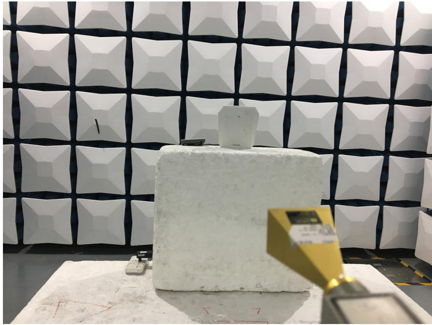
**Radiated Emissions (90GHz-100GHz) - Power supply by Adapter**
