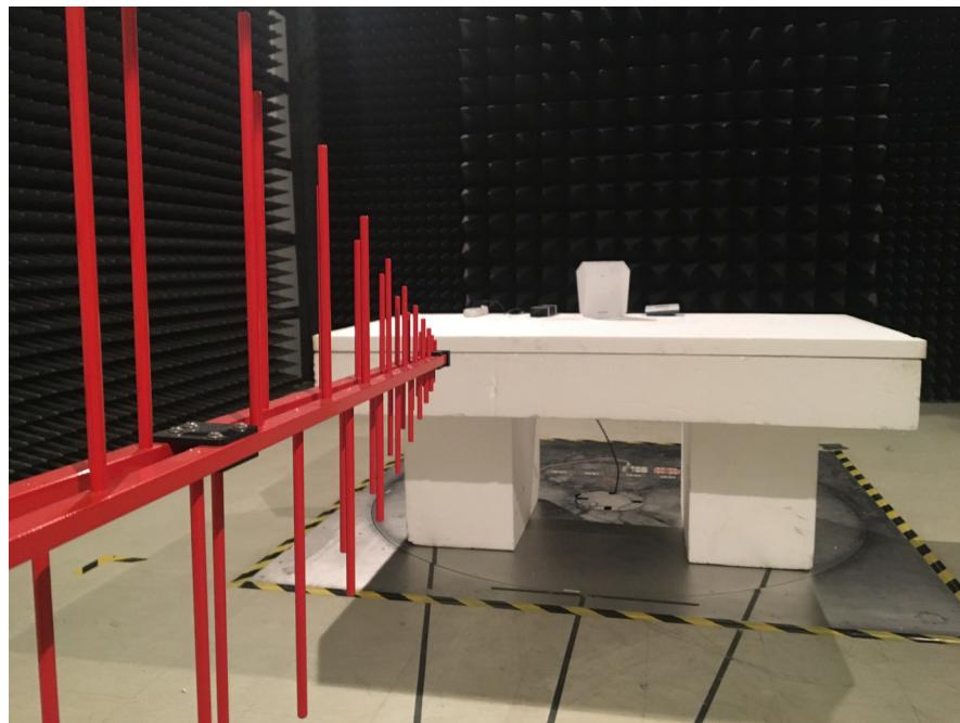
**Radiated Emissions (1GHz-18GHz) - Power supply by POE**
