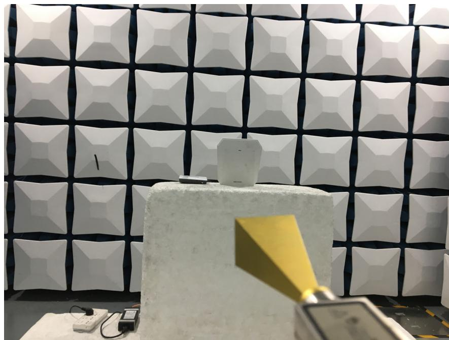
**Radiated Emissions (90GHz-100GHz) - Power supply by POE**
