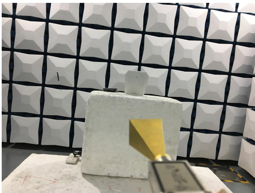
**Radiated Emissions (60GHz-75GHz) - Power supply by Adapter**
