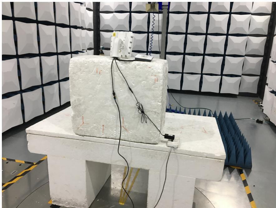
**Radiated Emissions (18GHz-40GHz) - Power supply by Adapter**
