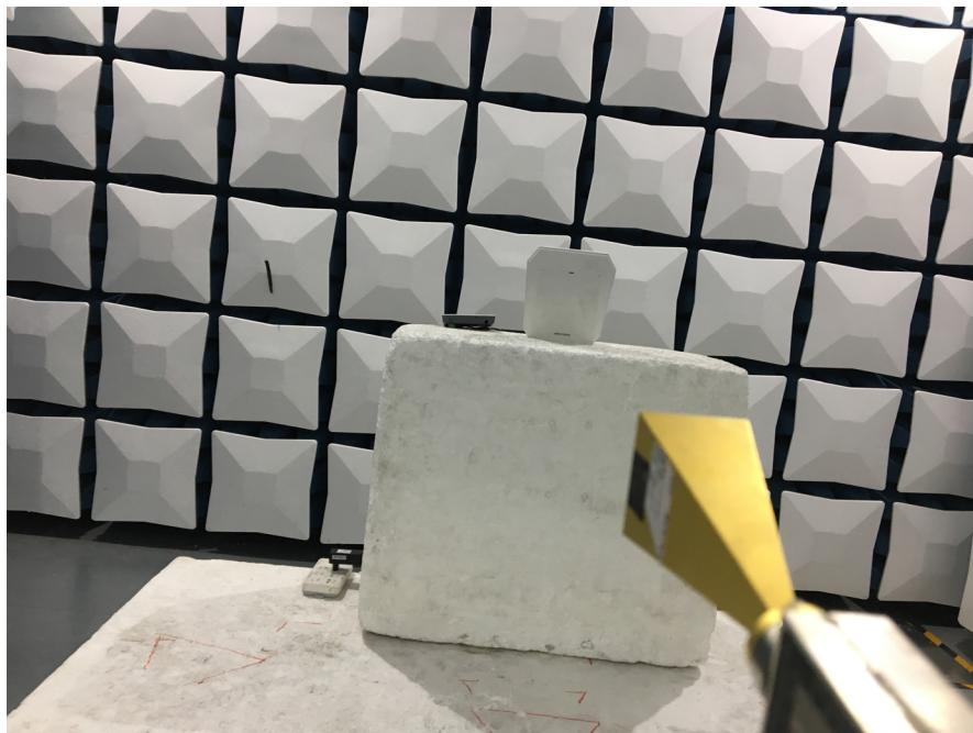
**Radiated Emissions (75GHz-90GHz) - Power supply by Adapter**
