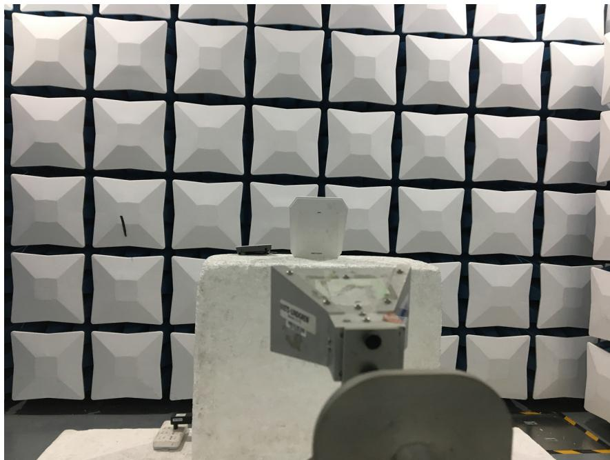
**Radiated Emissions (40GHz-60GHz) - Power supply by Adapter**
