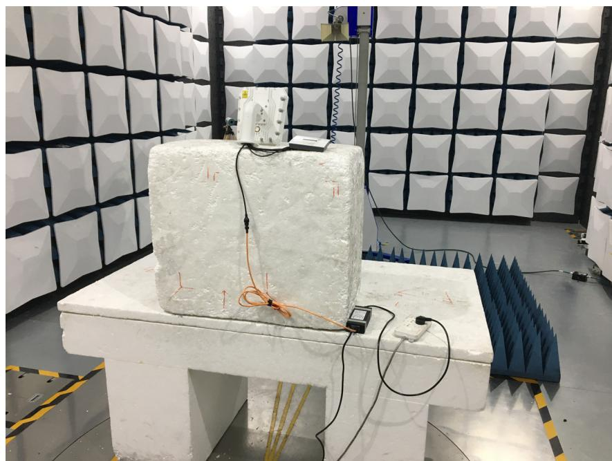
**Radiated Emissions (18GHz-40GHz) - Power supply by POE**
