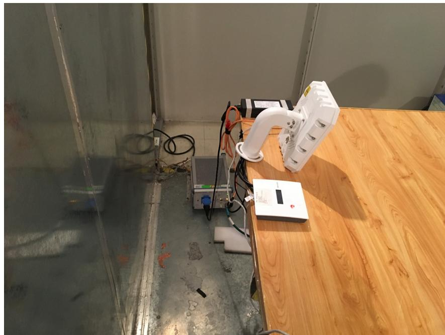
**Radiated Emissions (Below 1 GHz) - Power supply by POE**
