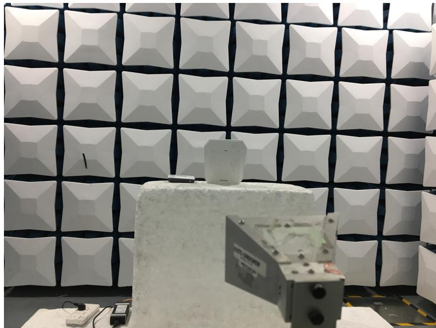
**Radiated Emissions (40GHz-60GHz) - Power supply by POE**
