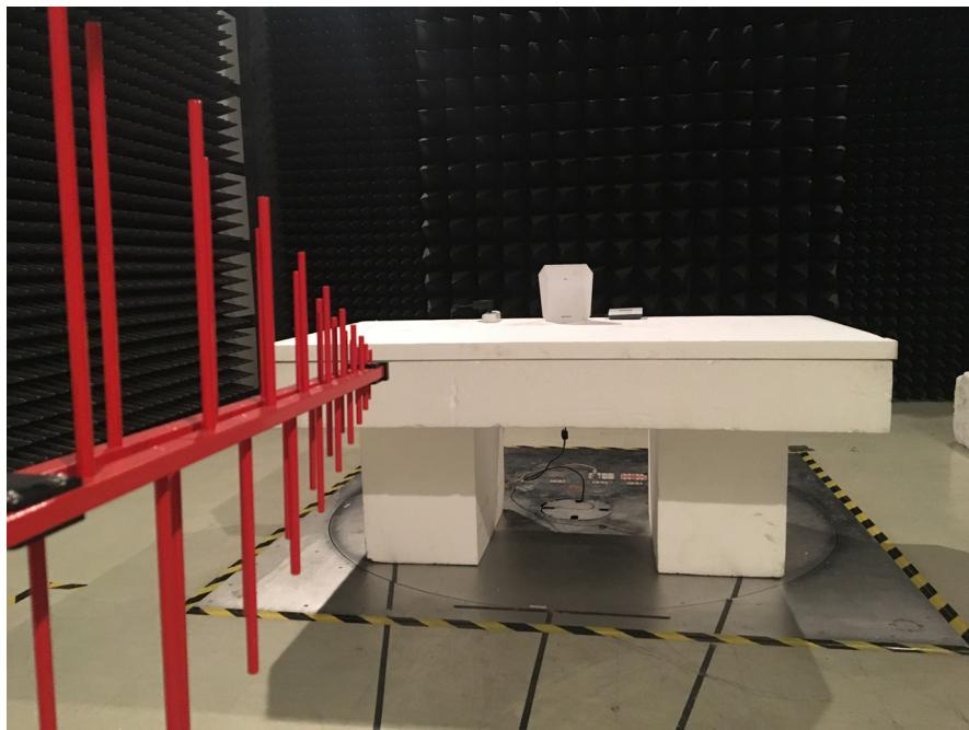
**Radiated Emissions (1GHz-18GHz) - Power supply by Adapter**
