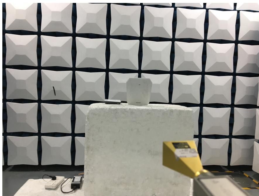
**Radiated Emissions (60GHz-75GHz) - Power supply by POE**
