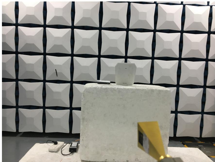
**Radiated Emissions (75GHz-90GHz) - Power supply by POE**
