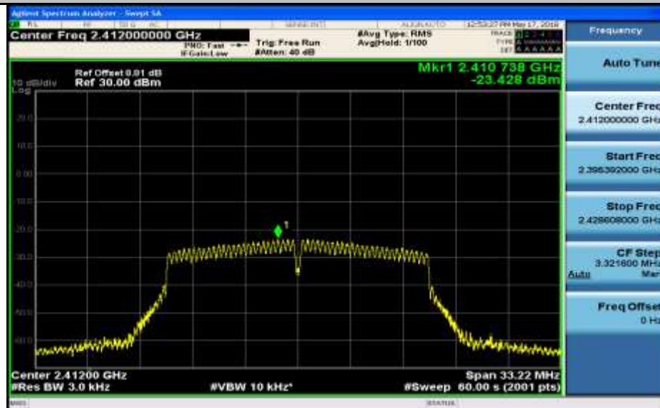
Maximum(average) power spectral density_11G_2437_Ant2
