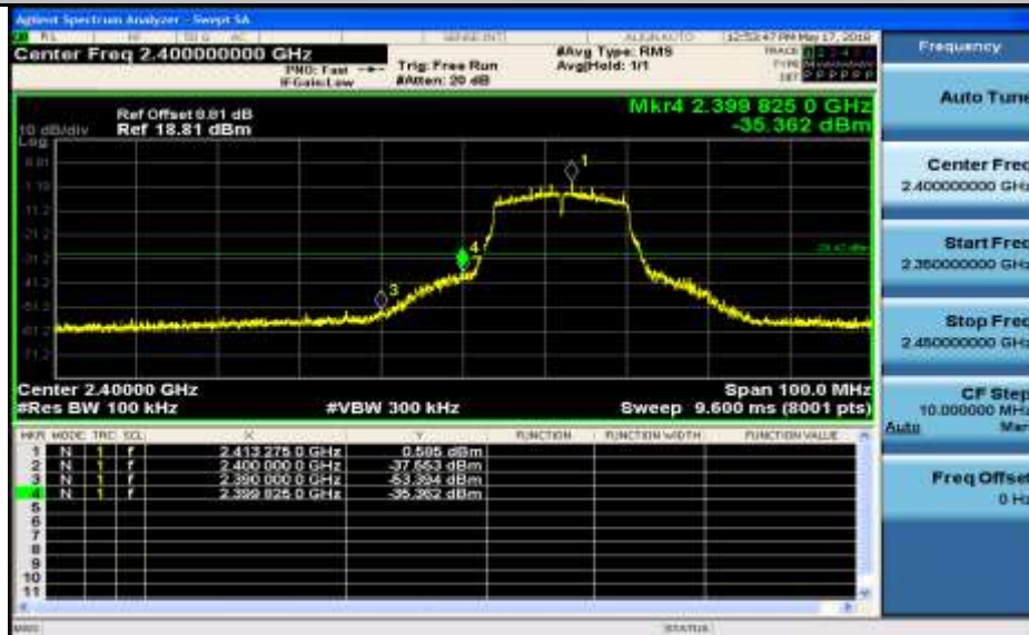
Band-edge for RF Conducted Emissions_11G_2412_Ant2
