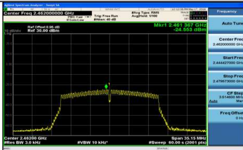
Maximum(average) power spectral density_11N20MIMO_2462_Ant1
