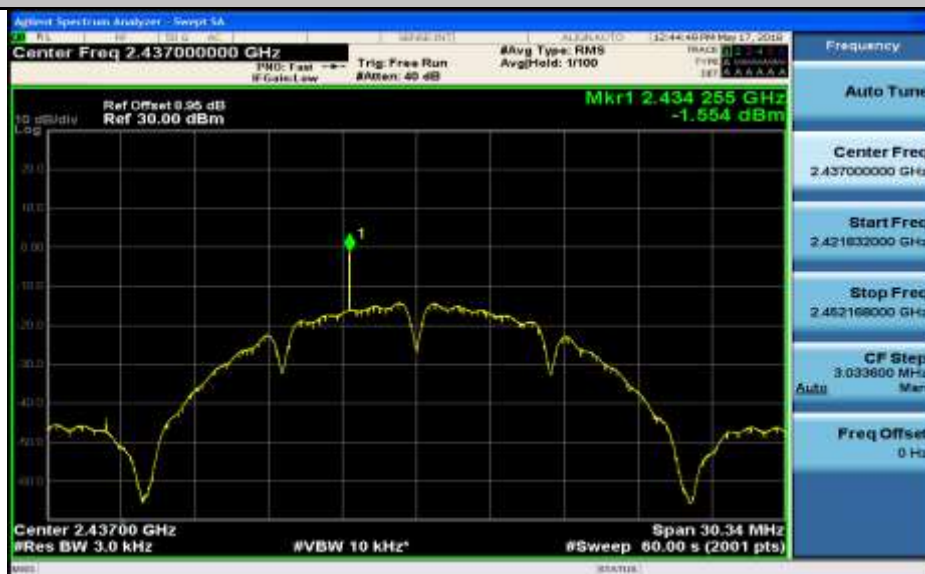
Maximum(average) power spectral density_11B_2462_Ant2
