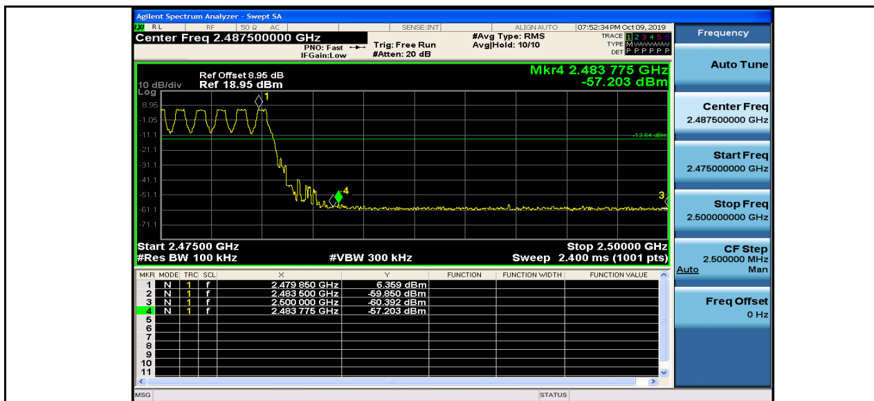
Band-edge for RF Conducted Emissions_DH5_2480_Hopping Off
