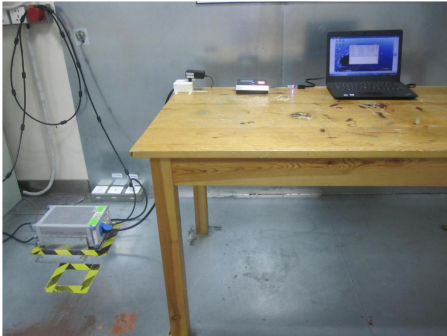
Photograph 1: Set-up for Conducted Emission on AC Mains
