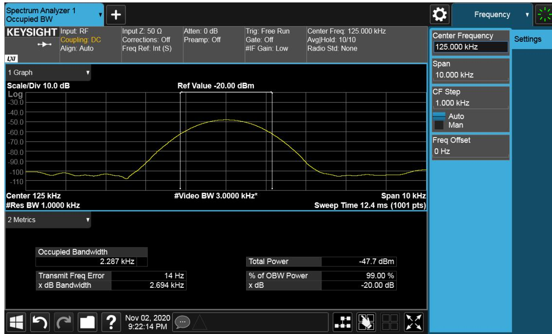
Remark: Because the measured signal is CW or CW-like adjusting the RBW per C63.10 would not be practical since measured bandwidth will always follow the RBW and the result will be approximately twice the RBW. And the signal was narrowband, therefore it was impossible to set RBW within 1% – 5%.
