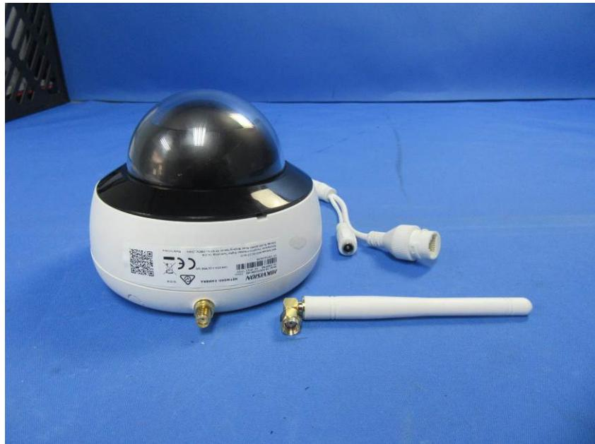
The Whip antenna is RP-SMA Connector and no consideration of replacement.
