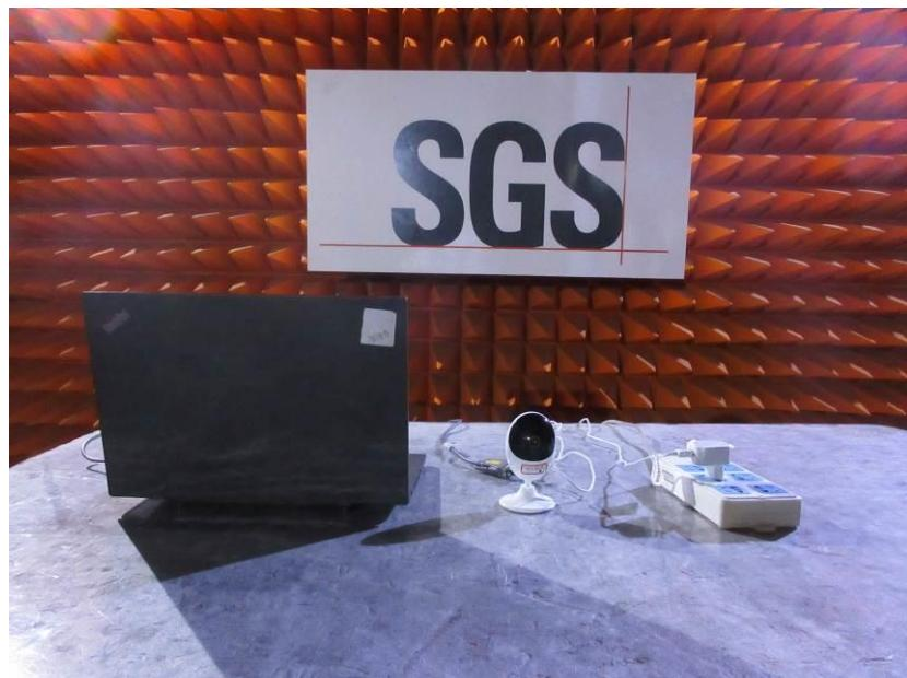
**2.3 RF Conducted Test Setup**
