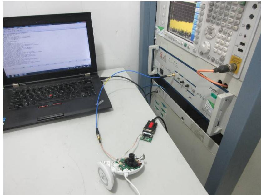
**2.3 Radiated Emission Test Setup**
