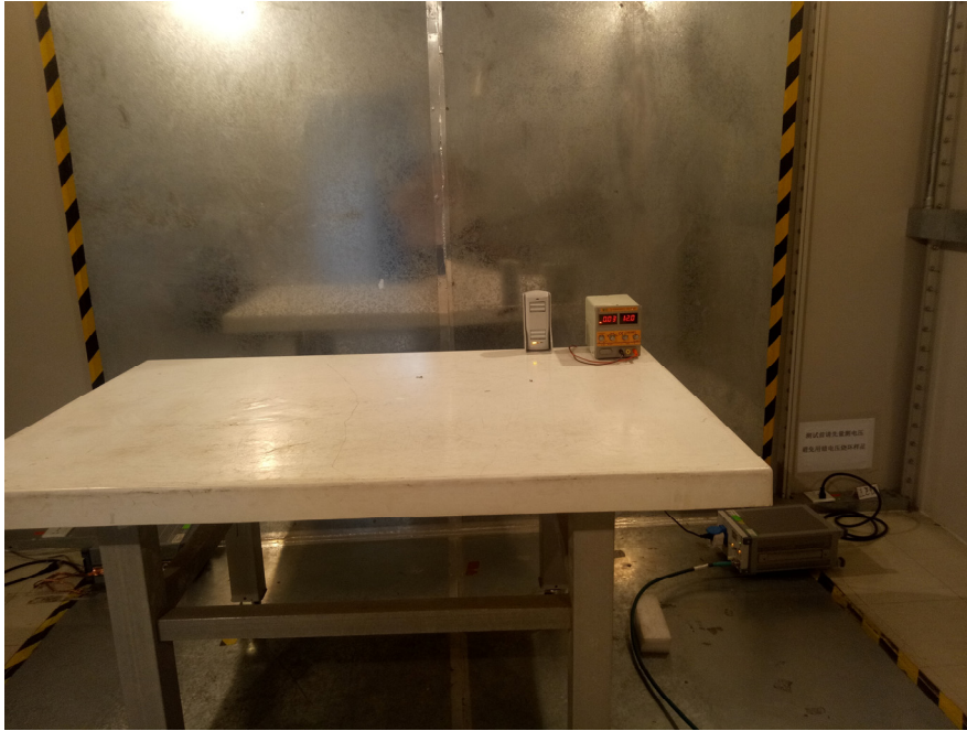
Conducted Emissions (Side View)
