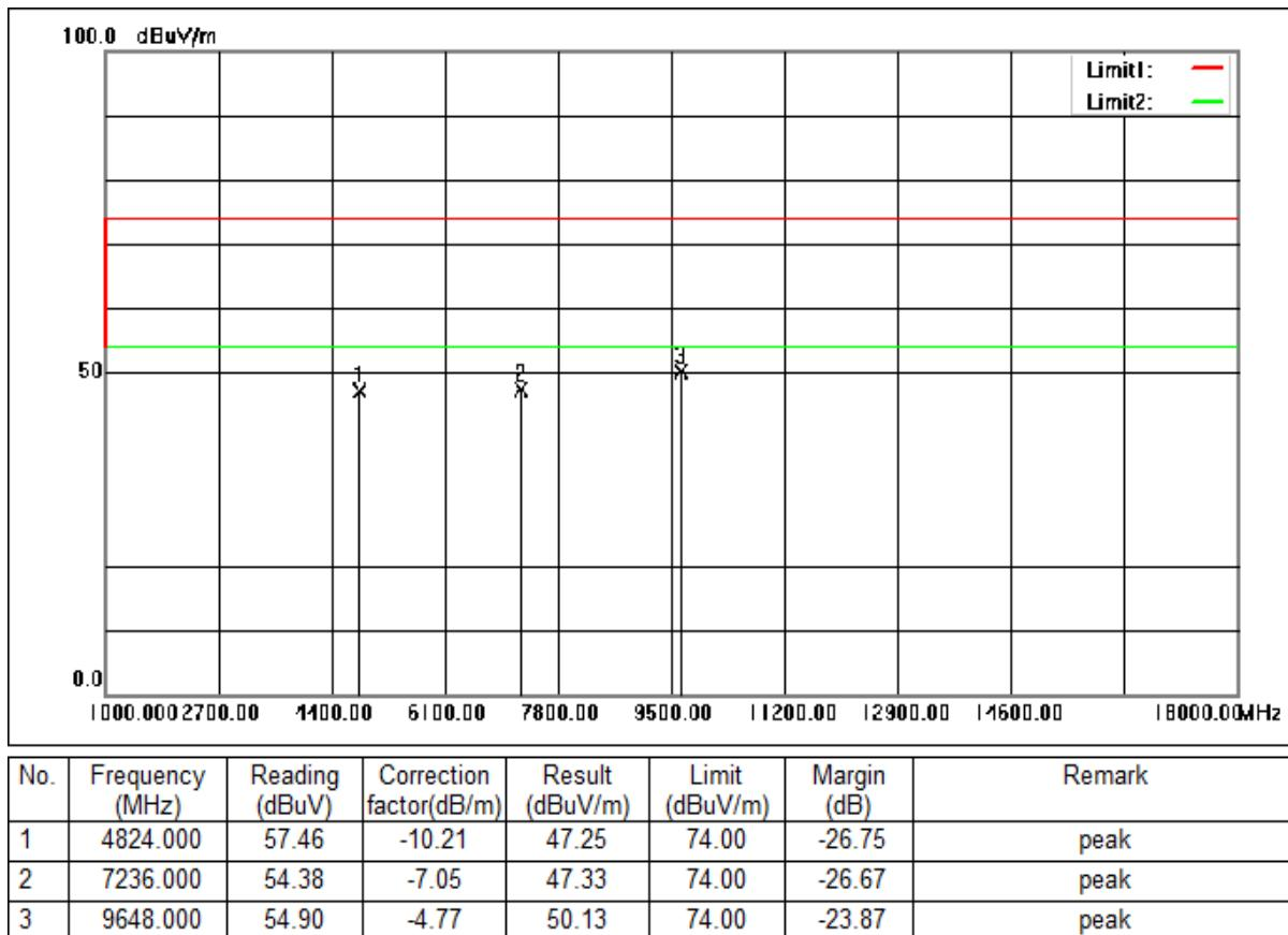
Mode:a; Polarization:Vertical; Modulation:b; bandwidth:20MHz; Channel:Low
