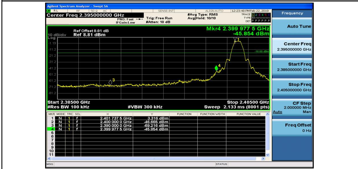
Band-edge for RF Conducted Emissions\_BLE\_2480\_Hopping Off
