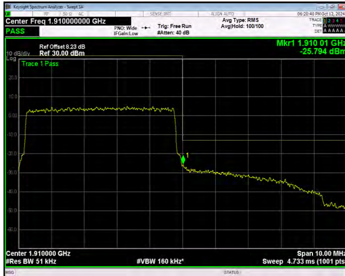
Band4 16QAM BW=1.4MHz Channel=19957 RB Size=1 Position=#0 Extended
