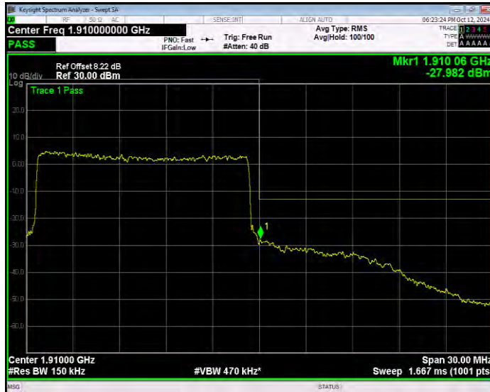
Band2 QPSK BW=20MHz Channel=18700 RB Size=1 Position=#0 Extended
