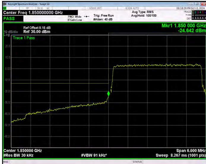
Band2 QPSK BW=3MHz Channel=19185 RB Size=1 Position=#0 Extended
