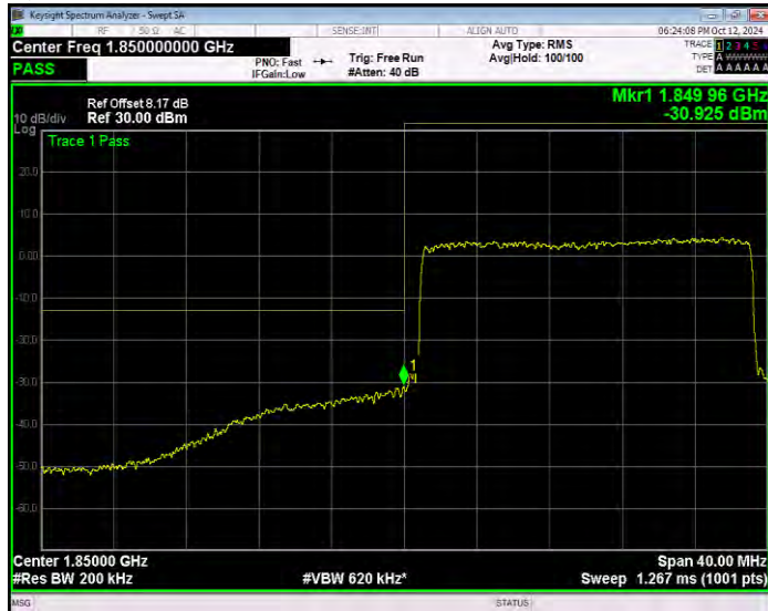
Band2 QPSK BW=20MHz Channel=19100 RB Size=1 Position=#0 Extended
