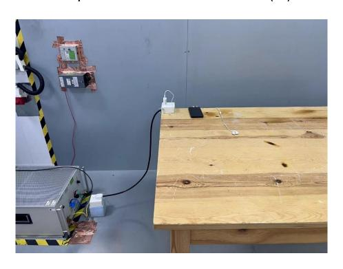
Set-up for Radiated Emission (RE), Below 1GHz
