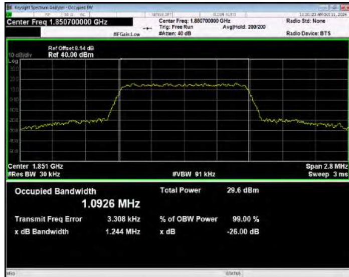
Band2 QPSK BW=1.4MHz Channel=18900 RB Size=6 Position=#0
