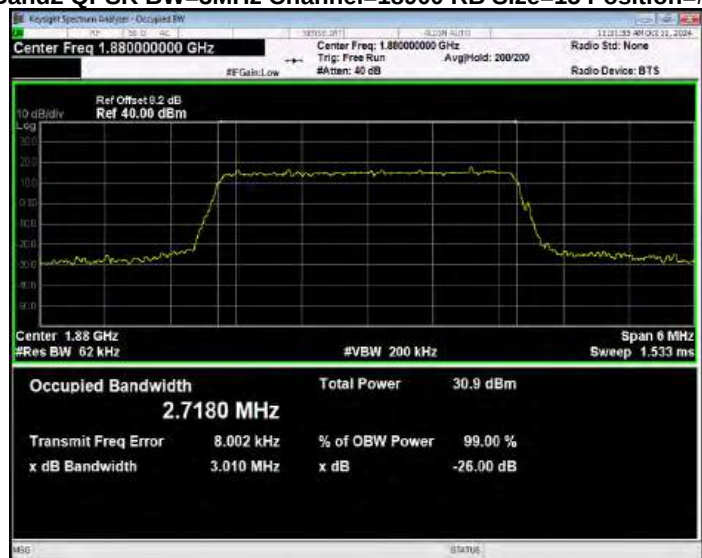
Band2 QPSK BW=3MHz Channel=19185 RB Size=15 Position=#0
