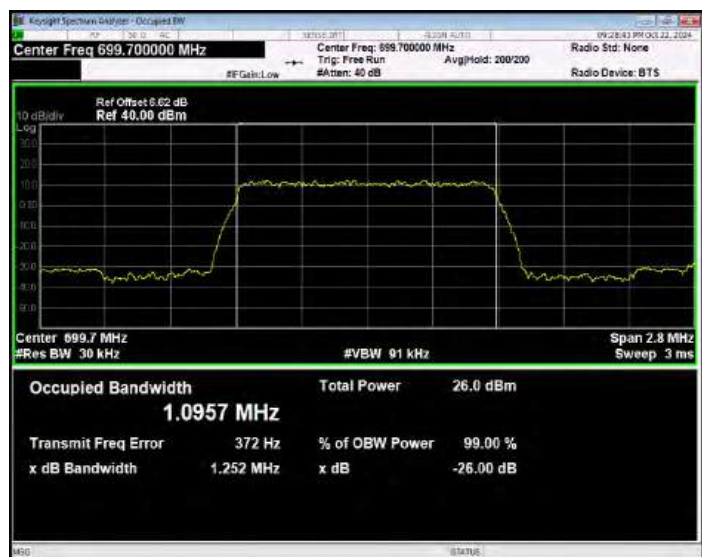
Band12 QPSK BW=1.4MHz Channel=23095 RB Size=6 Position=#0
