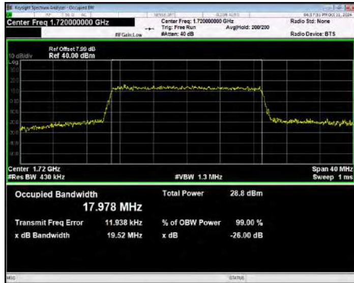
Band4 16QAM BW=20MHz Channel=20175 RB Size=100 Position=#0
