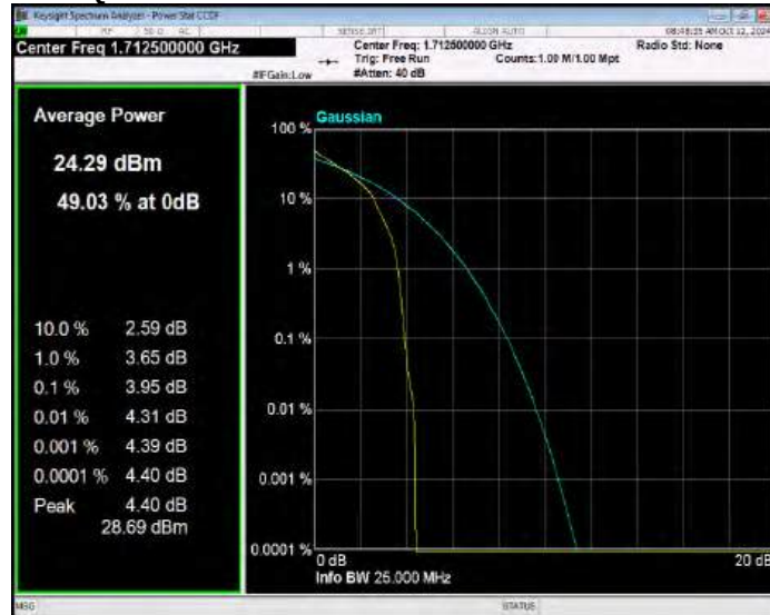
Band66 QPSK BW=5MHz Channel=132322 RB Size=1 Position=#0
