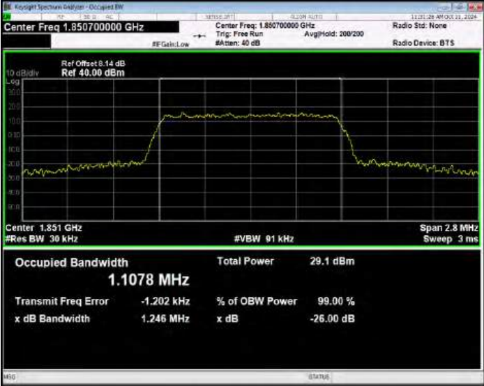
Band2 16QAM BW=1.4MHz Channel=18900 RB Size=6 Position=#0
