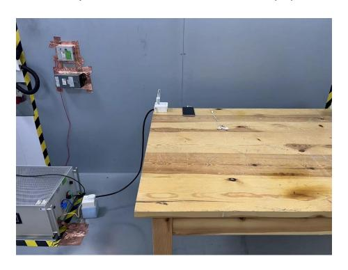
Set-up for Radiated Emission (RE), Below 1GHz
