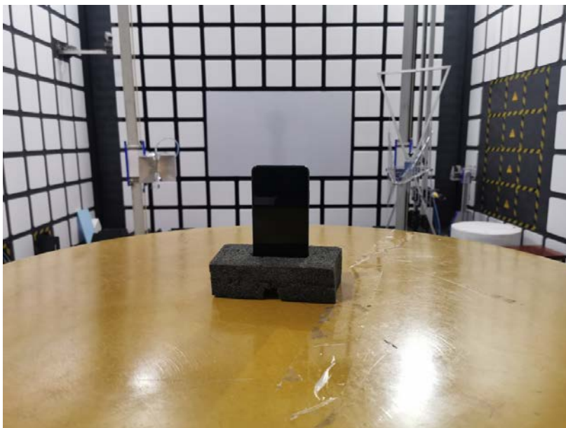
Spurious Radiated Emissions Test setup
