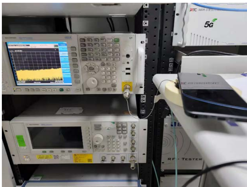
RF Conducted Test setup (BT/WIFI)
