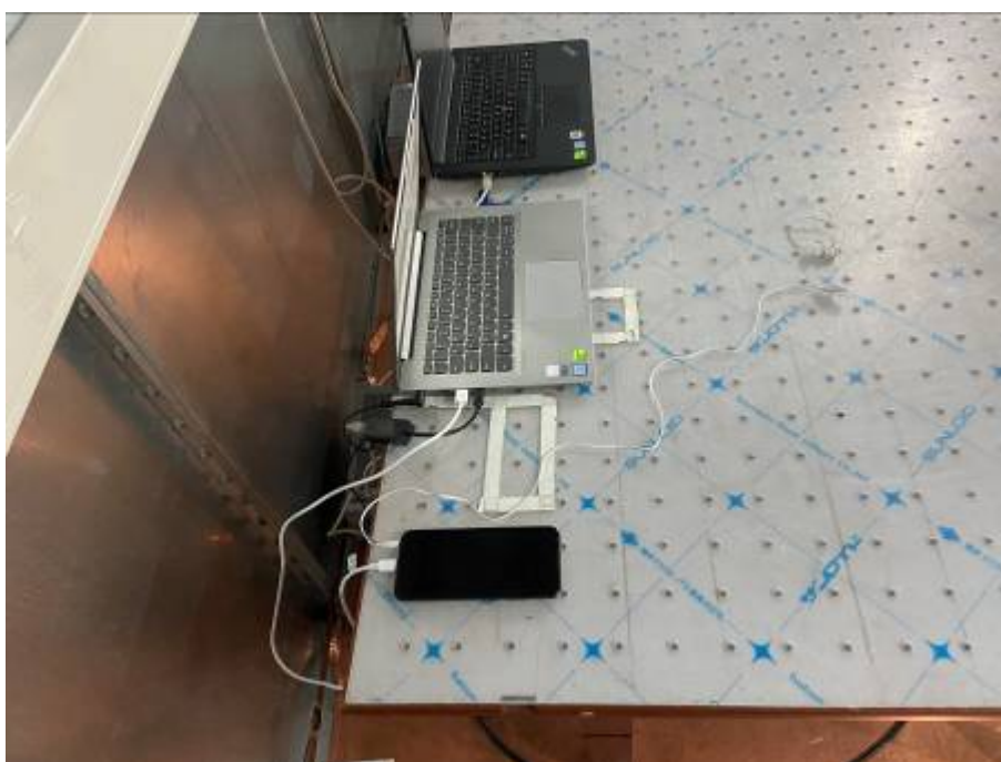
Conducted Emissions Test Setup (with laptop)
