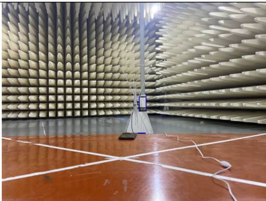
Radiated Emissions Test Setup (with charger) (30-1000MHz)
