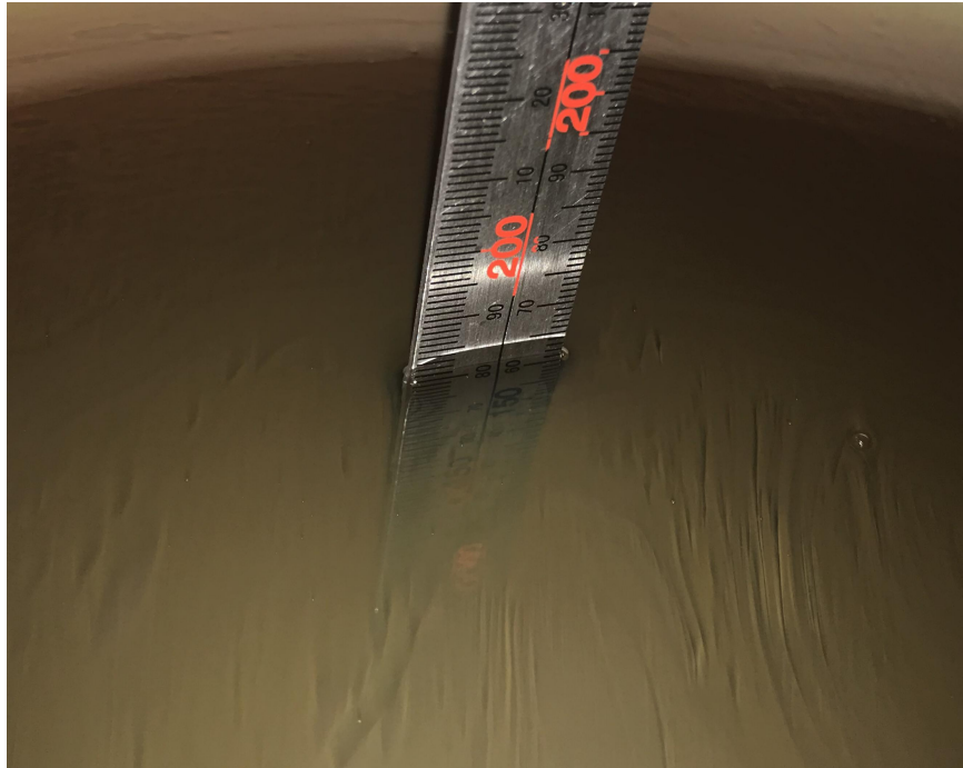
Liquid depth for SAR Measurement
