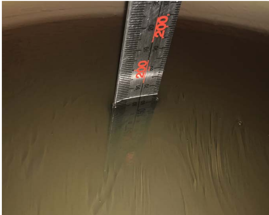
Liquid depth for SAR Measurement
