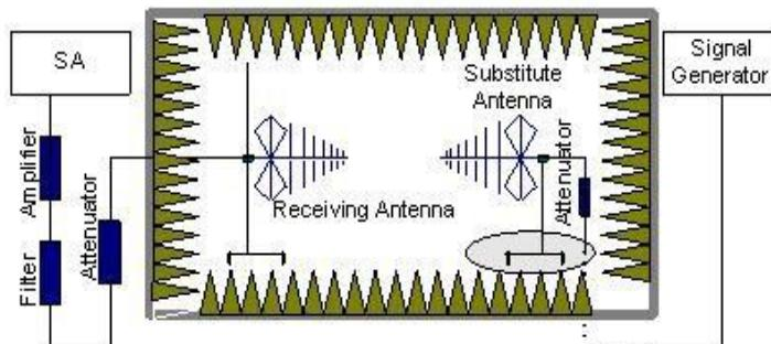
In the chamber, an substitution antenna for the frequency band of interest is placed at the
