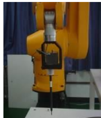
Picture C.2 Near-field Probe
