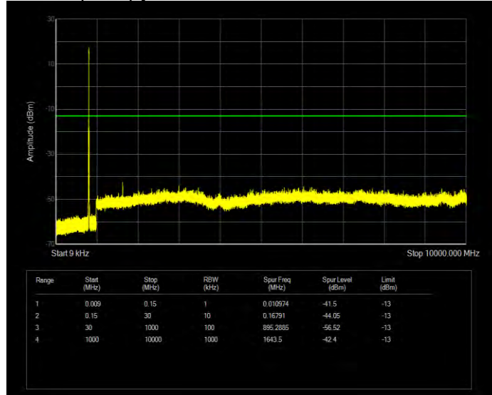
Band26(814-824) QPSK BW=5MHz Channel=26715 RB Size=25 Position=#0
