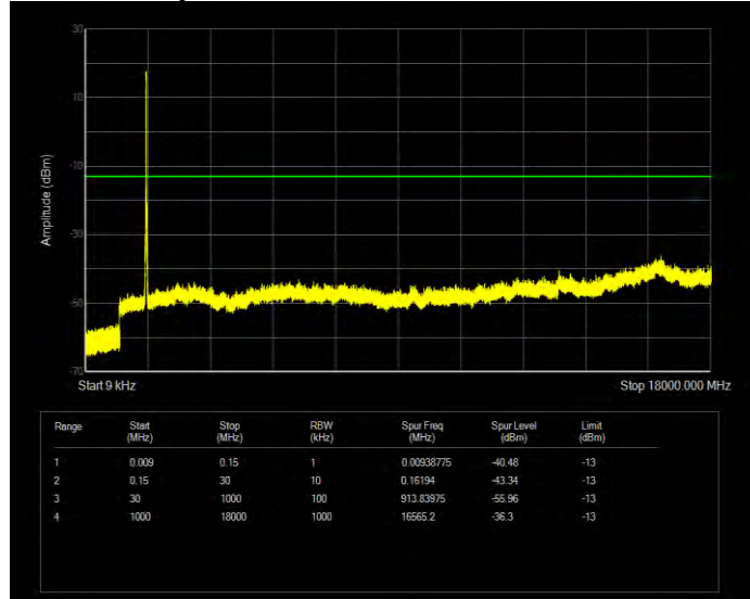
Band66 16QAM BW=20MHz Channel=132072 RB Size=100 Position=#0
