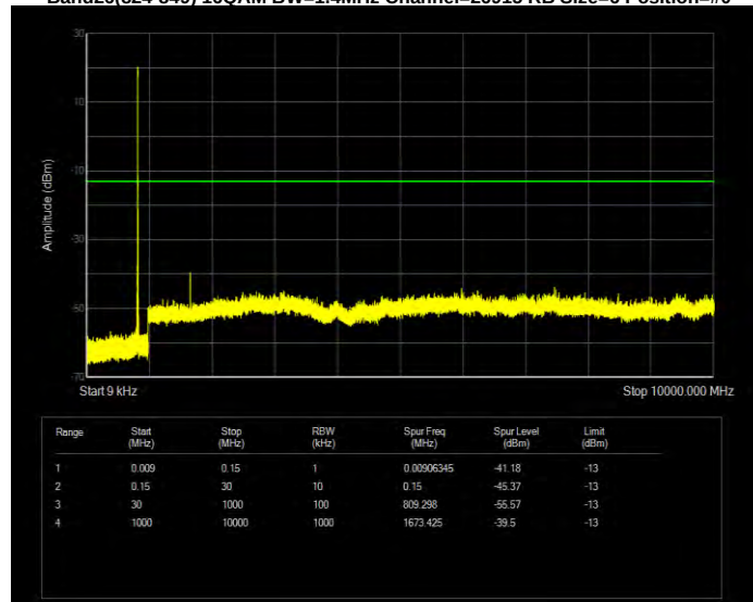
Band26(824-849) 16QAM BW=1.4MHz Channel=26915 RB Size=6 Position=#0
