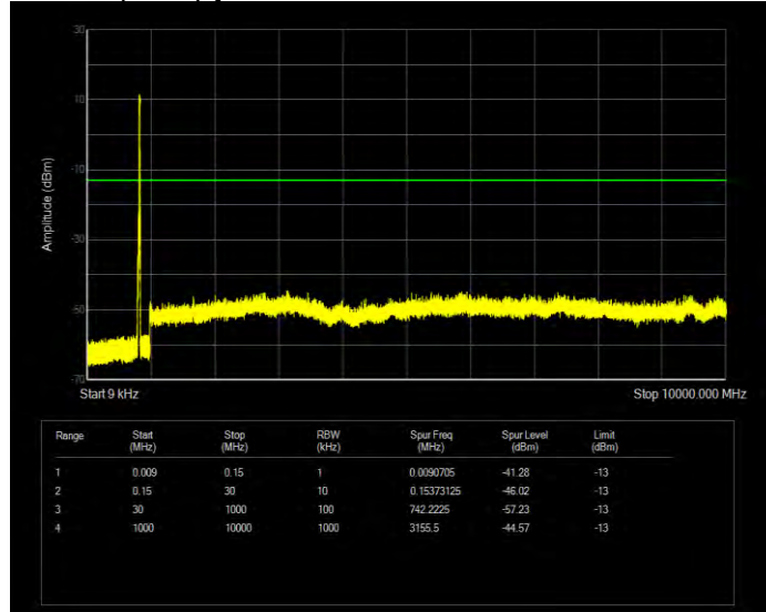
Band26(824-849) QPSK BW=3MHz Channel=26805 RB Size=15 Position=#0
