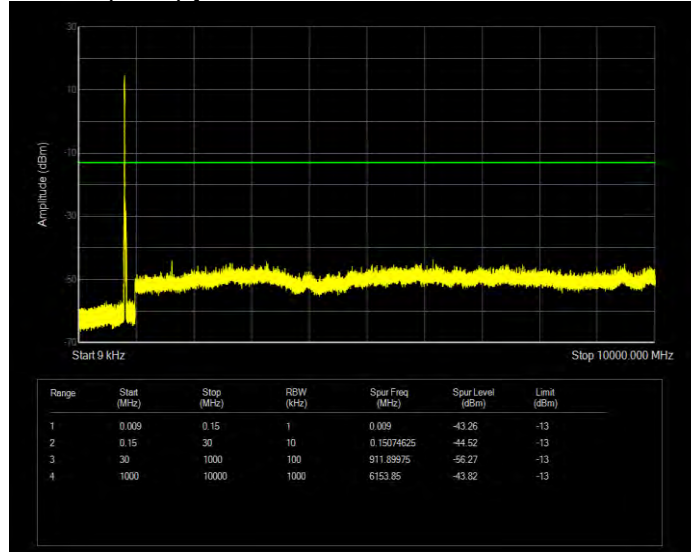
Band26(814-824) QPSK BW=3MHz Channel=26705 RB Size=15 Position=#0
