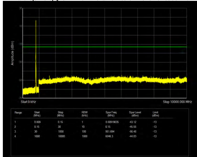
Band26(824-849) QPSK BW=5MHz Channel=26915 RB Size=25 Position=#0
