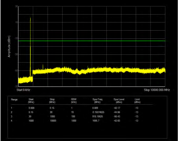
Band26(824-849) QPSK BW=1.4MHz Channel=26797 RB Size=6 Position=#0
