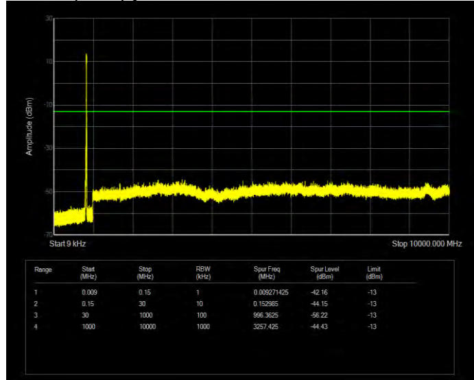
Band26(824-849) QPSK BW=15MHz Channel=26865 RB Size=75 Position=#0
