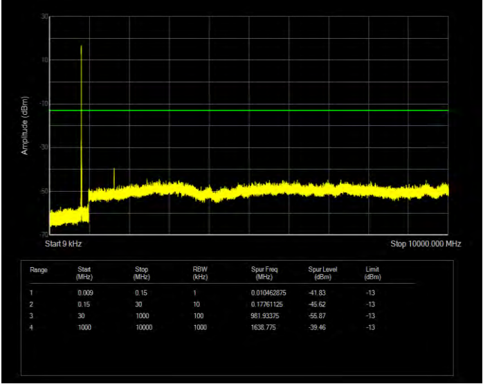
Band26(814-824) 16QAM BW=3MHz Channel=26775 RB Size=15 Position=#0
