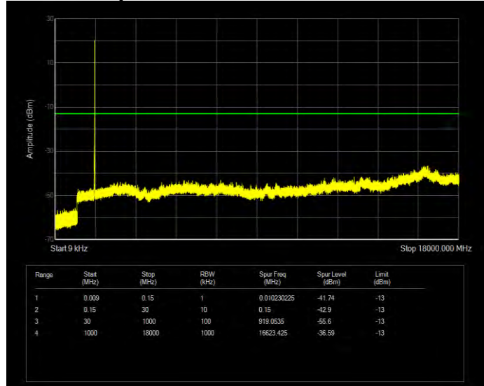
Band66 QPSK BW=1.4MHz Channel=131979 RB Size=6 Position=#0
