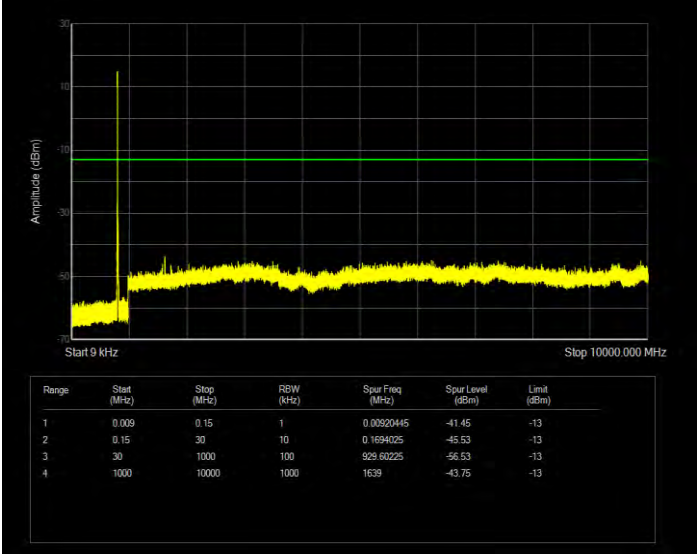
Band26(814-824) 16QAM BW=5MHz Channel=26765 RB Size=25 Position=#0
