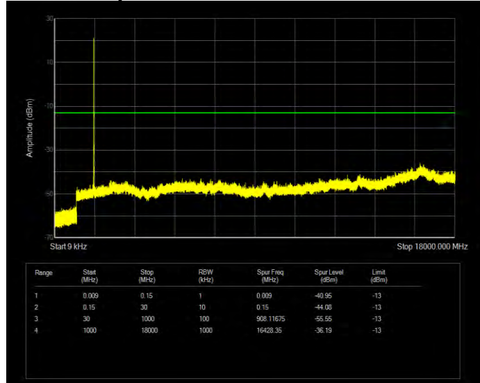
Band66 16QAM BW=5MHz Channel=131997 RB Size=25 Position=#0
