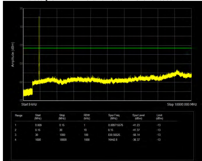
Band66 QPSK BW=5MHz Channel=132322 RB Size=25 Position=#0
