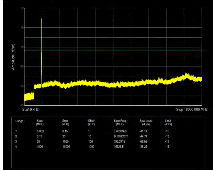
Band66 16QAM BW=15MHz Channel=132047 RB Size=75 Position=#0
