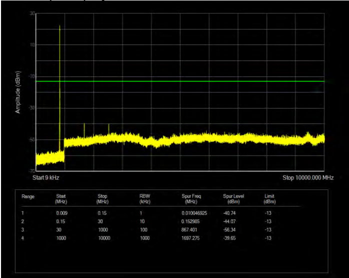
Band26(824-849) 16QAM BW=10MHz Channel=26840 RB Size=50 Position=#0
