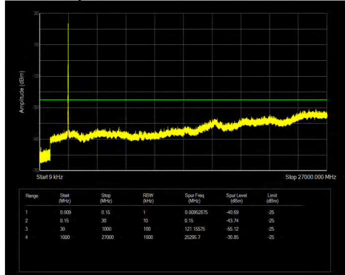
Band41 QPSK BW=15MHz Channel=39725 RB Size=75 Position=#0
