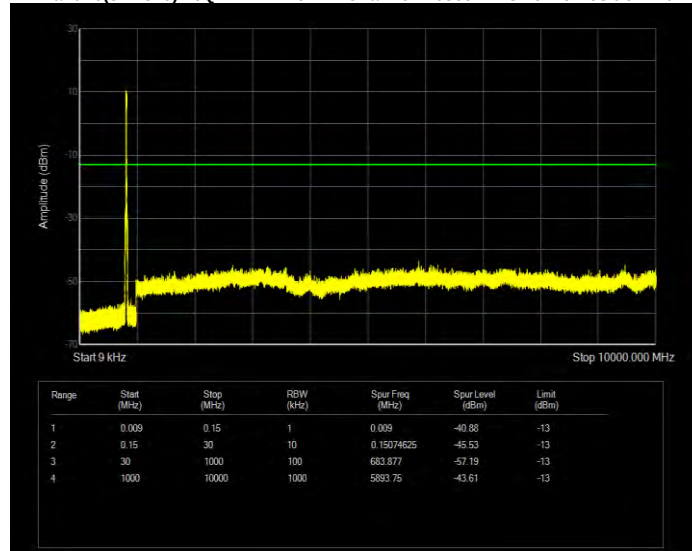
Band26(824-849) 16QAM BW=15MHz Channel=26915 RB Size=75 Position=#0
