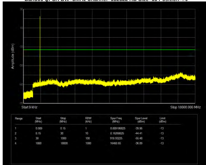
Band66 QPSK BW=3MHz Channel=132322 RB Size=15 Position=#0
