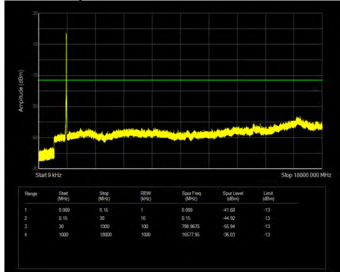
Band66 16QAM BW=3MHz Channel=131987 RB Size=15 Position=#0
