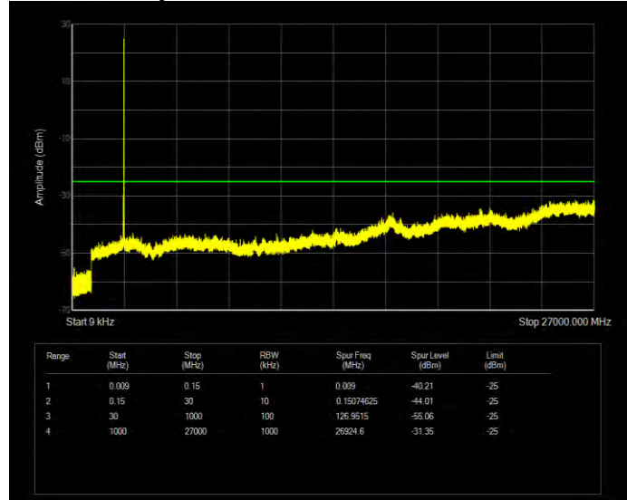
Band41 QPSK BW=10MHz Channel=39700 RB Size=50 Position=#0
