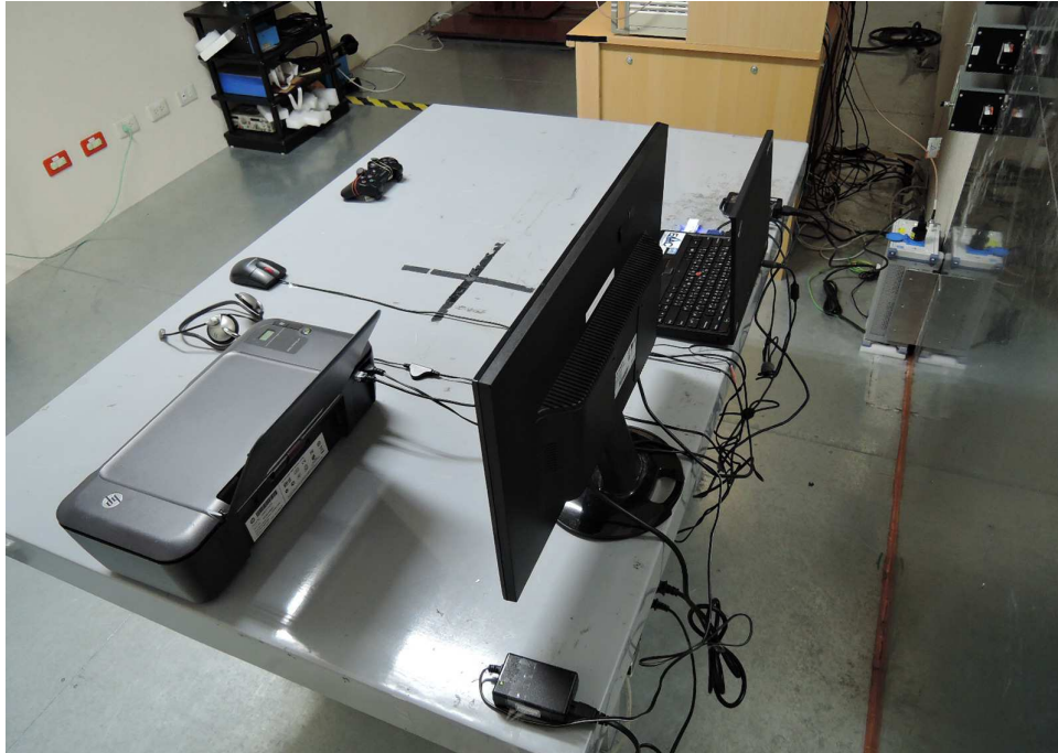
Photograph 5: Set-up for for Mains Conducted testing Back
