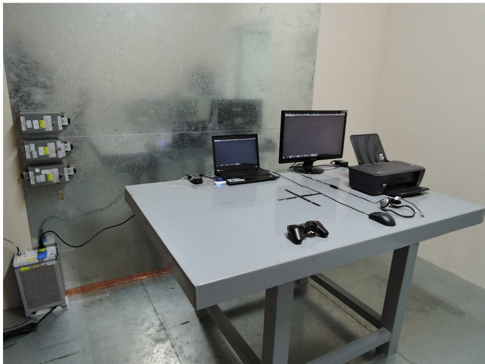
Photograph 6: Set-up for for Mains Conducted testing Front
