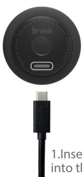
1. Insert the cable into the USB-C port
