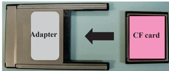
**Note:** Keep a card horizontal when inserting it into a card slot. An inclined card causes a failure.
