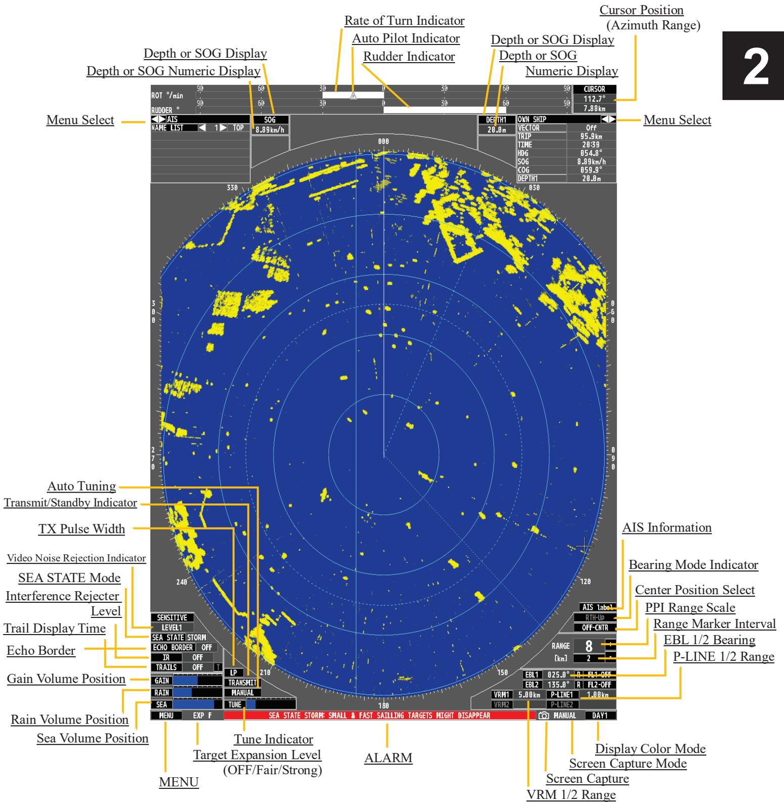
FIG 2.1 DISPLAY & READOUTS
