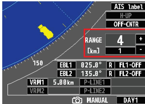
In this case, the distance interval of The Range Rings is 1km.
