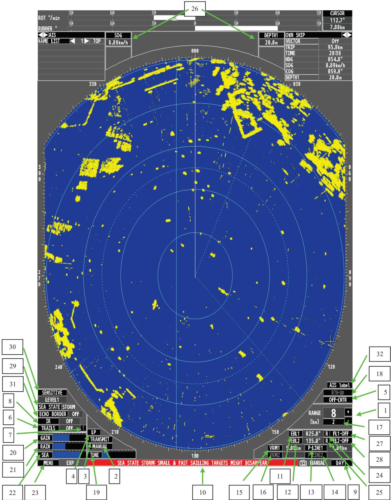
Fig 2.3 On-screen controls
