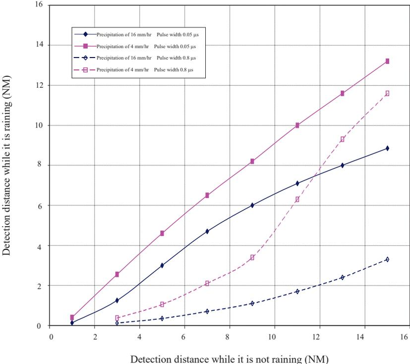
Figure 5.4 Decreased target detection distance due to precipitation
