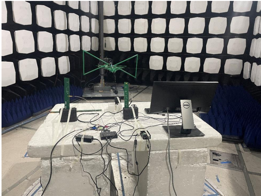
Figure 7 – Test Set up Rear View - Radiated Emissions <1 GHz – Four Antennas
