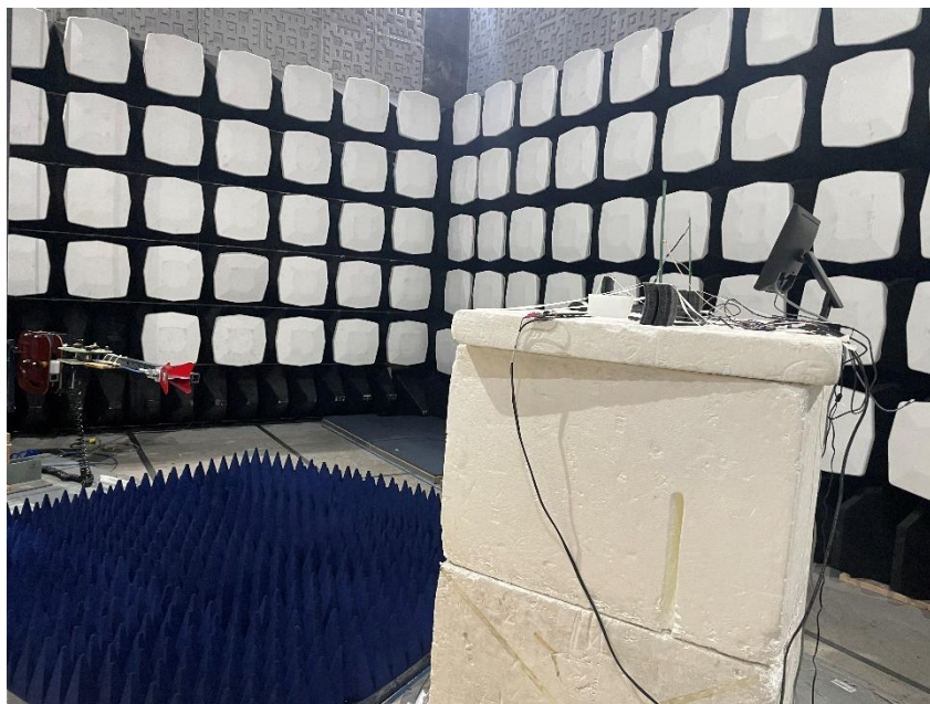
Figure 11 – Test Set up Rear View - Radiated Emissions <10 GHz – Four Antennas
