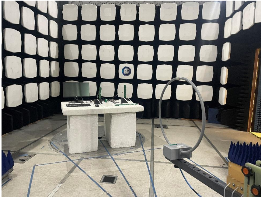
Figure 1 – Test Set up Front View - Radiated Emissions <30 MHz – Four Antennas
