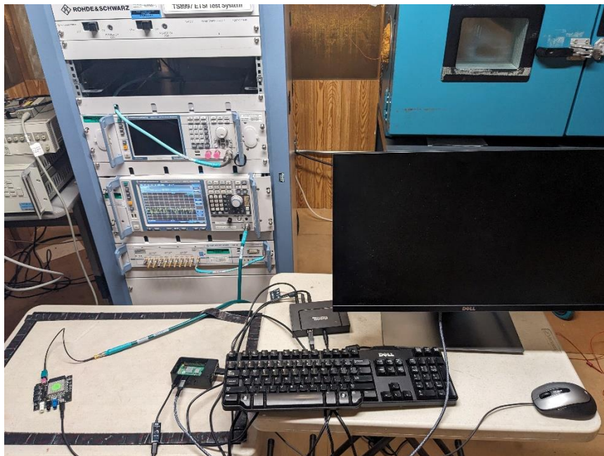
Figure 14 – Test Set up – Antenna Port Measurement
