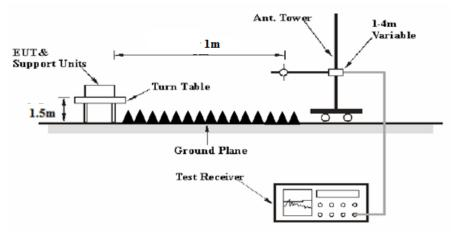
The radiated emission Below 1GHz tests were performed in the 3 meters chamber test site A, above 1GHz tests were performed in the 3 meters chamber test site B, using the setup accordance with the ANSI C63.10-2013. The specification used was the FCC 15.209, and FCC 15.407 limits.
