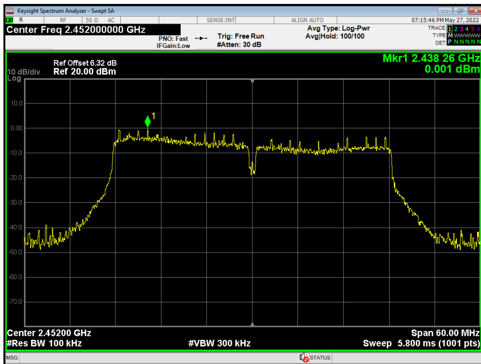
Tx. Spurious NVNT ax40 2452MHz Ant1 Emission
