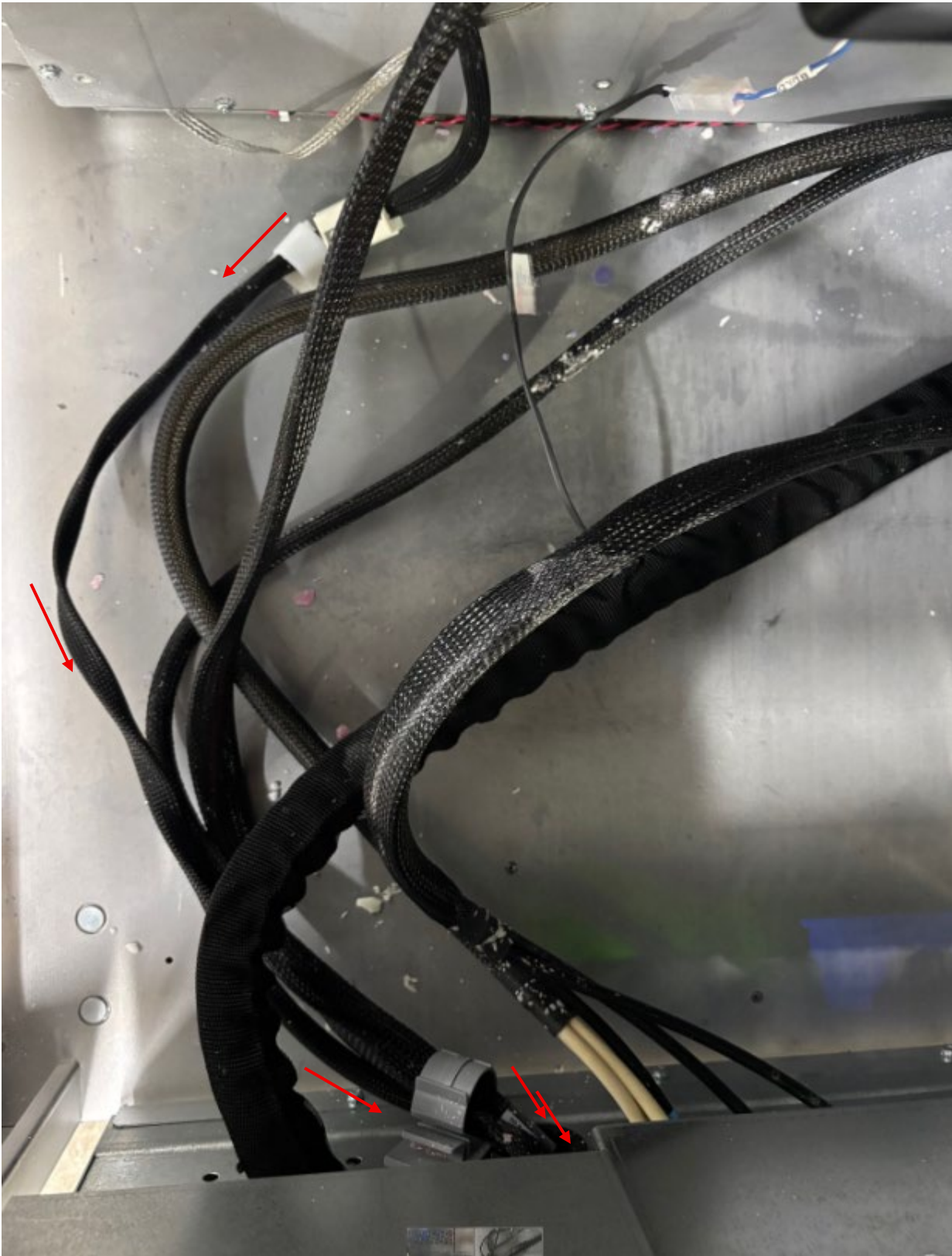
RFID cable routed to Material Delivery Drawer. Top view
