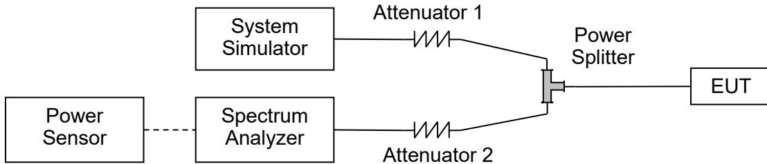
The EUT is coupled to the Spectrum Analyzer (SA) and the System Simulator (SS) with Attenuators through the Power Splitter; the RF load attached to the EUT antenna terminal is 50Ohm; the path loss as the factor is calibrated to correct the reading. The EUT is commanded by the SS to operate at the maximum output power. A call is established between the EUT and the SS.
