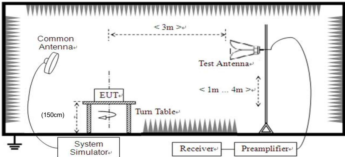
The EUT is located in a 3m Full-Anechoic Chamber; the cable loss, air loss and so on of the site as factors are pre-calibrated using the "Substitution" method, and calculated to correct the reading.
