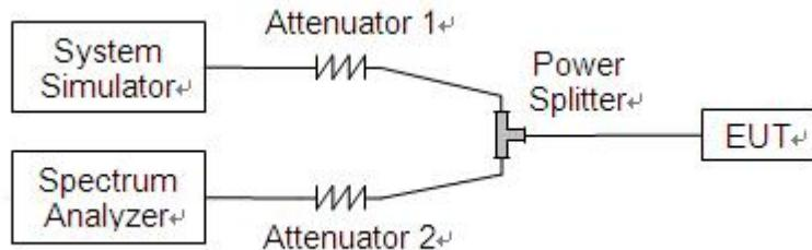
The EUT is coupled to the Spectrum Analyzer (SA) and the System Simulator (SS) with Attenuators through the Power Splitter; the RF load attached to the EUT antenna terminal is 50Ω; the path loss as the factor is calibrated to correct the reading. The EUT is commanded by the SS to operate at the maximum output power i.e. Power Control Level (PCL) = 5 and Power Class = 4. A call is established between the EUT and the SS.
