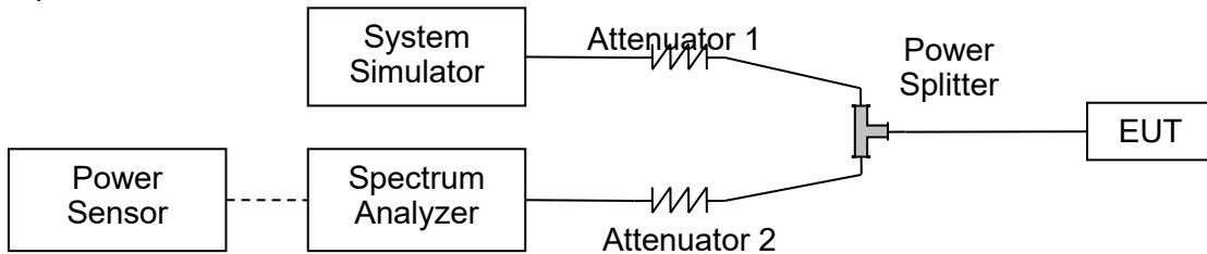
The EUT is coupled to the Spectrum Analyzer (SA) and the System Simulator (SS) with Attenuators through the Power Splitter; the RF load attached to the EUT antenna terminal is 50Ohm; the path loss as the factor is calibrated to correct the reading. The EUT is commanded by the SS to operate at the maximum output power i.e. Power Control Level (PCL) = 5 and Power Class = 4. A call is established between the EUT and the SS.
