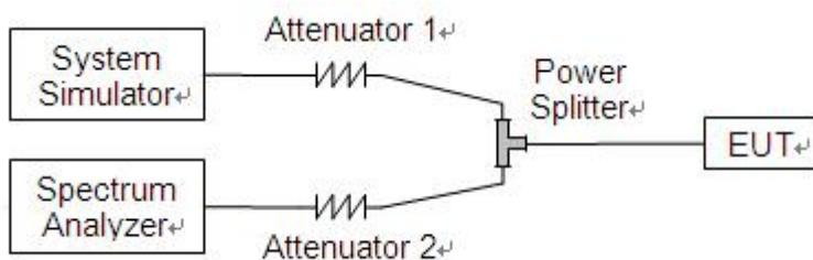
The EUT is coupled to the Spectrum Analyzer (SA) and the System Simulator (SS) with Attenuators through the Power Splitter; the RF load attached to the EUT antenna terminal is 50 Ohm; the path loss as the factor is calibrated to correct the reading. The EUT is commanded by the SS to operate at the maximum output power i.e. Power Control Level (PCL) = 5 and Power Class = 4. A call is established between the EUT and the SS.
