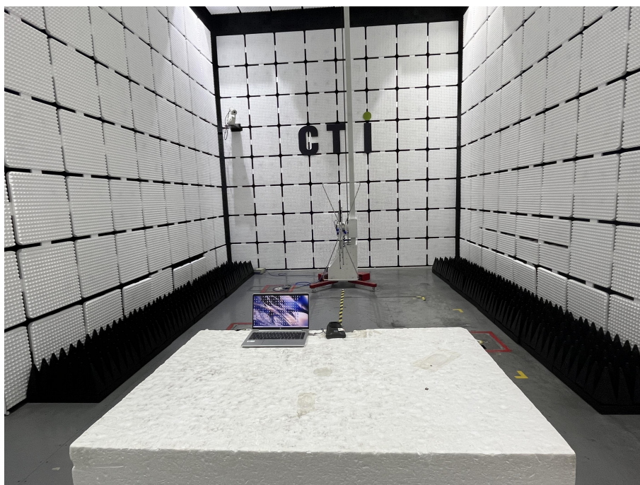
Radiated spurious emission Test Setup-1(Below 1GHz)
