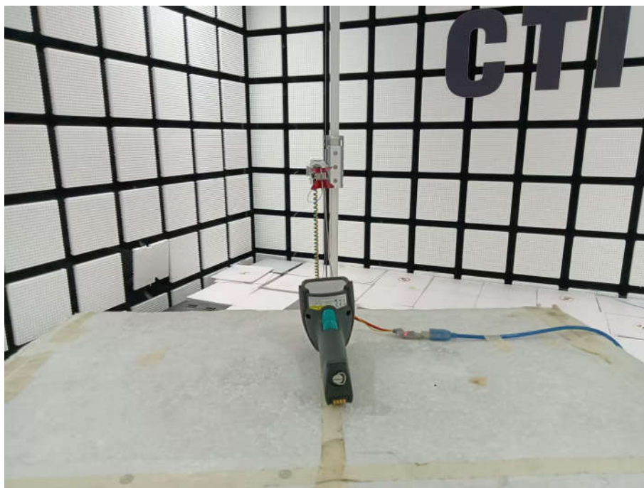
Radiated spurious emission Test Setup-2(Above 1GHz)
