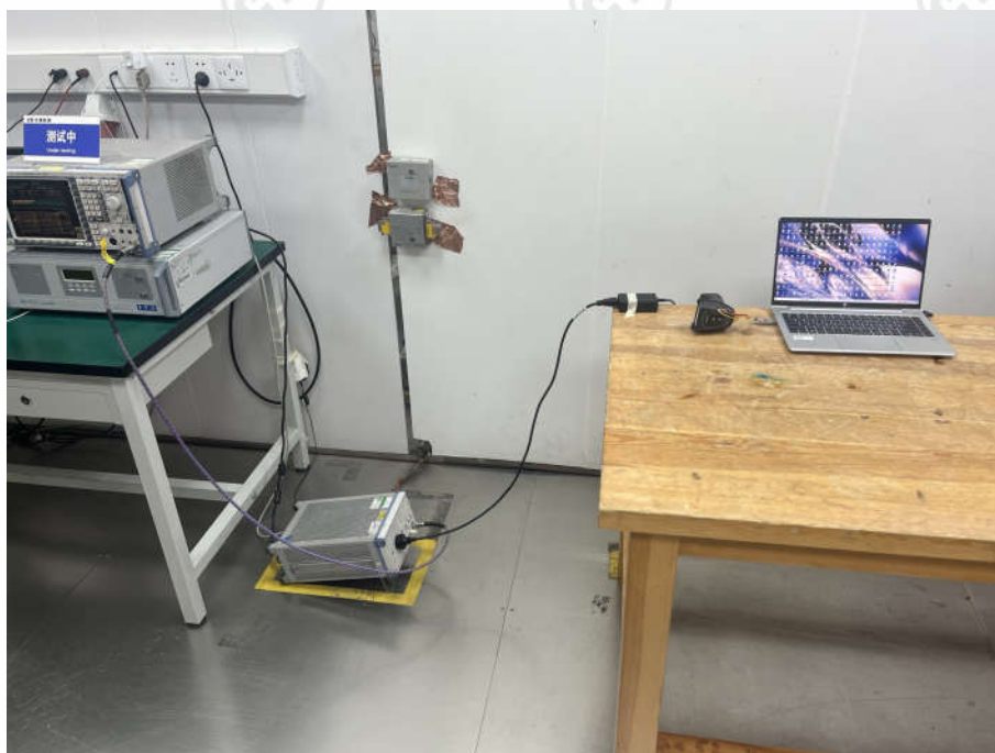
Conducted Emissions Test Setup
