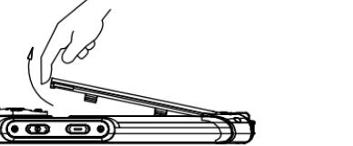
3. Insert the battery into the compartment per the illustrated direction, then press it tightly
