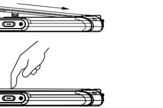
5. Slide the battery cover latch towards the left to lock the cover
