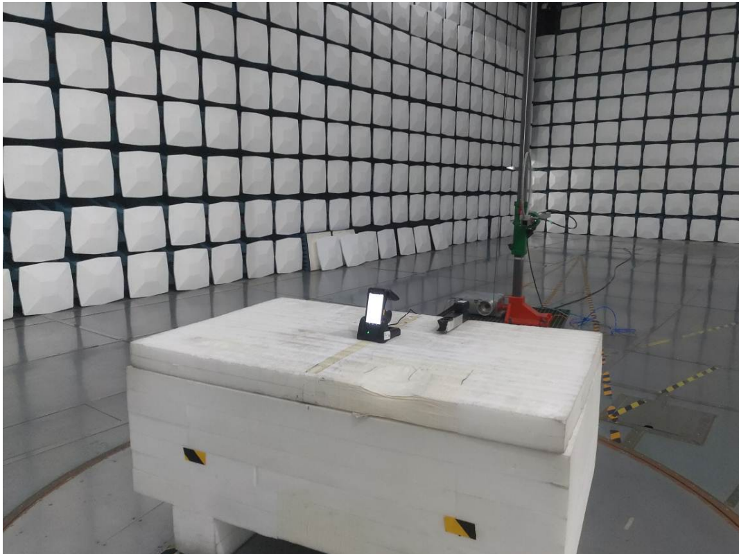
Radiated Emission 9k-30MHz Perpendicular View
