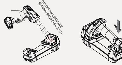
Note: The laser center needs to be aligned with the barcode center
