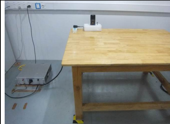
Conducted Emissions Test Setup Front View
