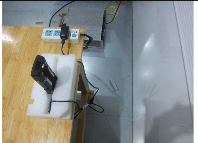
Conducted Emissions Test Setup Side View
