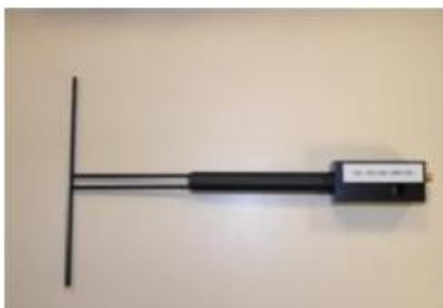
Figure 1 – Satimo COMOSAR Validation Dipole
