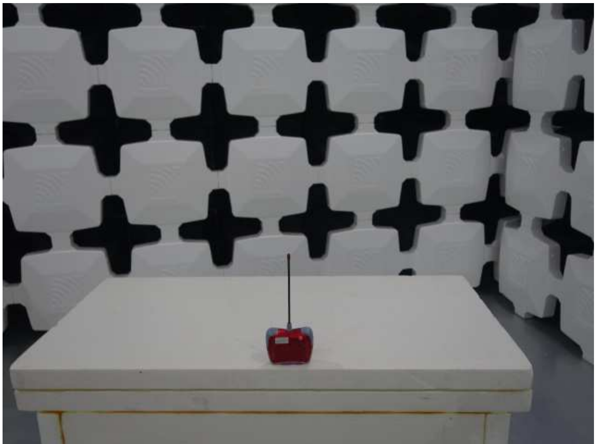
(The EUT placed in the centre of the turntable)
