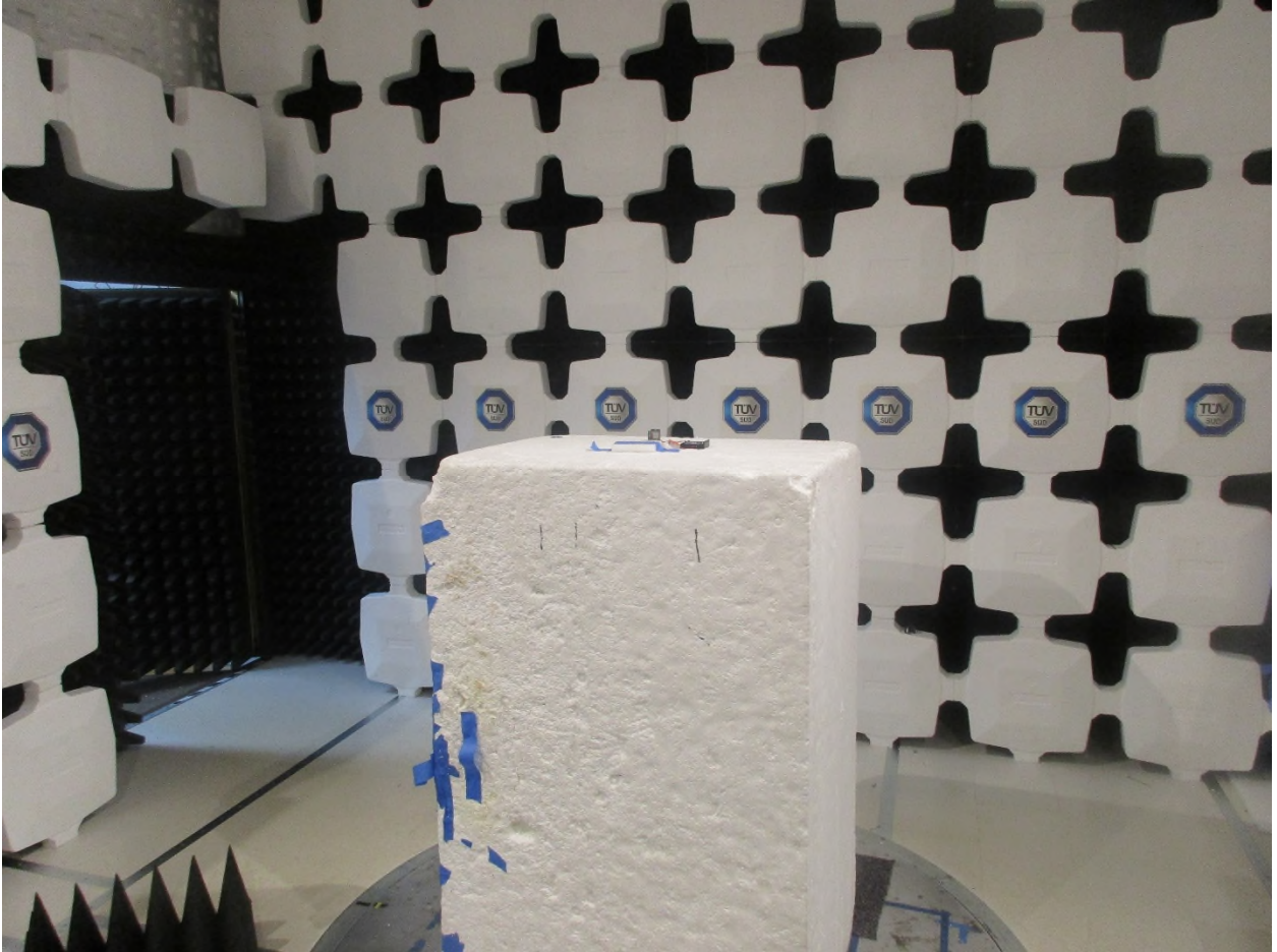
Figure 17: Radiated Emissions – Front View – Chip Antenna
