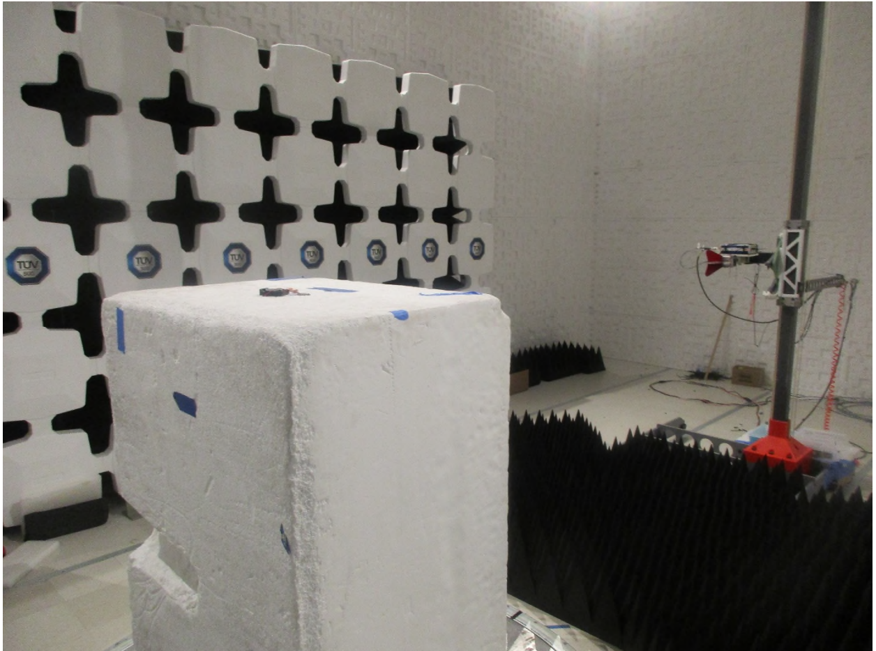
Figure 6: Radiated Emissions – Back View – PCB Trace Antenna
