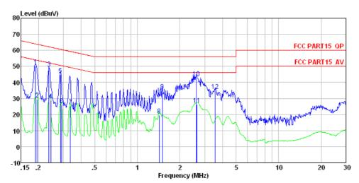
Condition : FCC PART15 QP LISN-2013 LINE EUT : Bluetooth Speaker Model : YB-801 Test Mode : Operating + Charging mode Power Rating : AC 120V/60Hz Test Engineer: David
