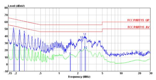
Condition : FCC PART15 QP LISN-2013 NEUTRAL EUT : Bluetooth Speaker Model : YB-801 Test Mode : Operating + Charging mode Power Rating : AC 120V/60Hz Test Engineer: David
