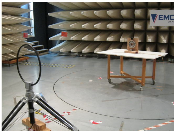
Radiated emissions measurement at 3 m distance in semi anechoing chamber (SAC) 9 kHz – 30 MHz
