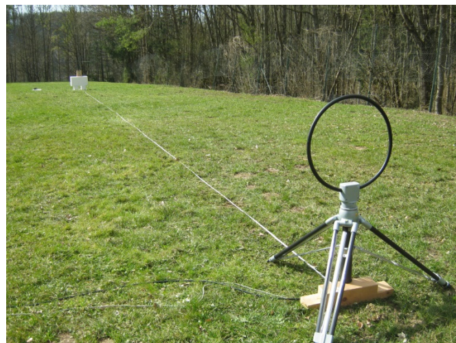
Radiated emissions measurement at 30 m distance at open area test site 9 kHz – 30 MHz
