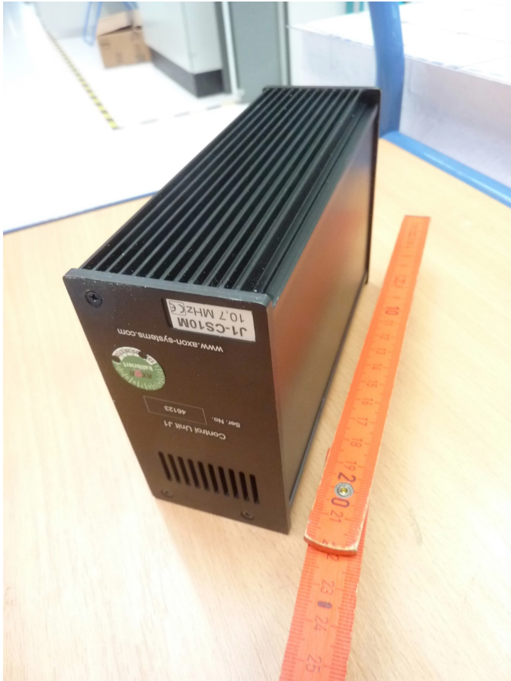
3 D view 2 AXON Systems Control Unit J1
