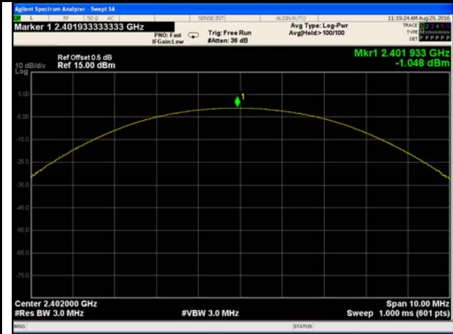
8DPSK Output power - Low CH 2402
