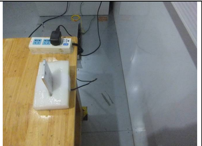
Conducted Emissions Test Setup Side View
