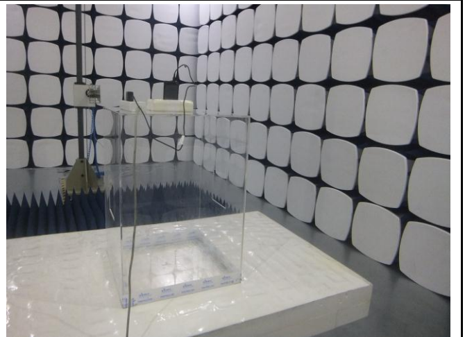
Radiated Spurious Emissions Test Setup Above 1GHz
