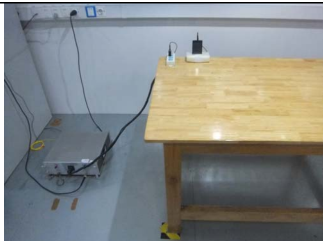
Conducted Emissions Test Setup Front View
