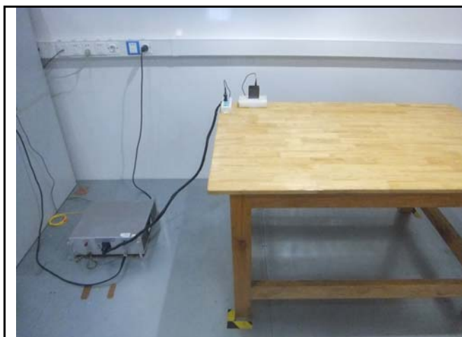
Conducted Emissions Test Setup Front View
