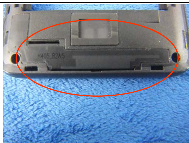
GSM/PCS/UMTS-FDD Antenna View
