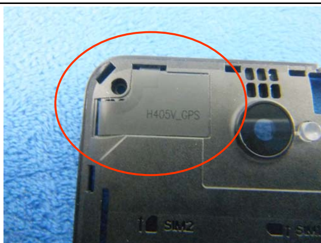
WIFI/BT/BLE/GPS - Antenna View
