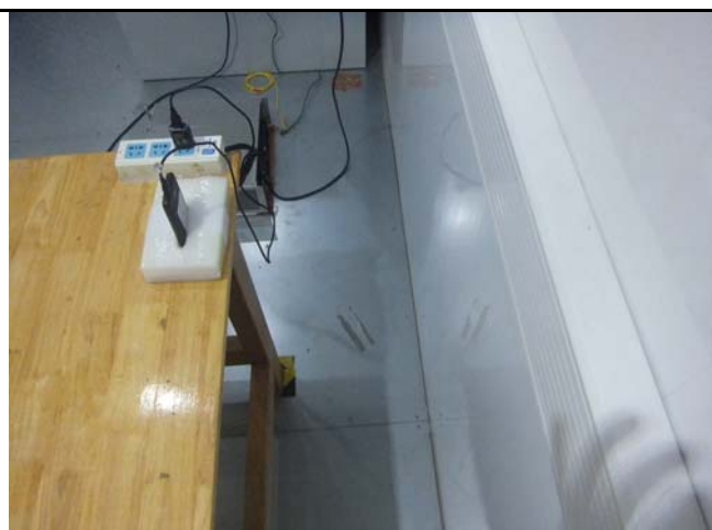
Conducted Emissions Test Setup Side View
