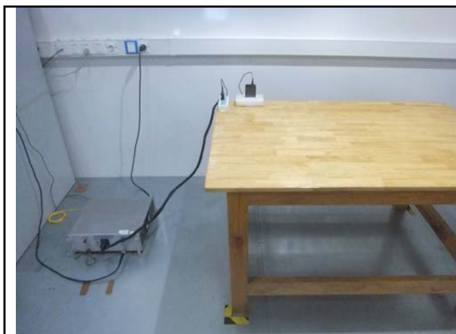
Conducted Emissions Test Setup Front View
