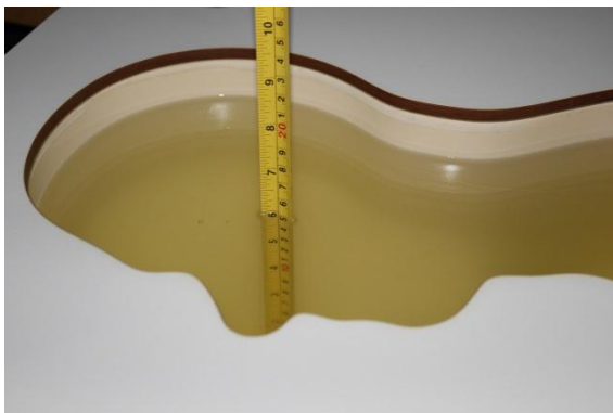
Liquid depth in the head phantom (1750MHz)
