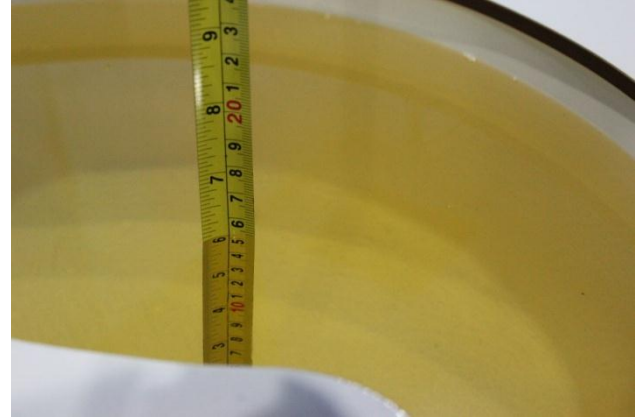
Liquid depth in the body phantom (750MHz)
