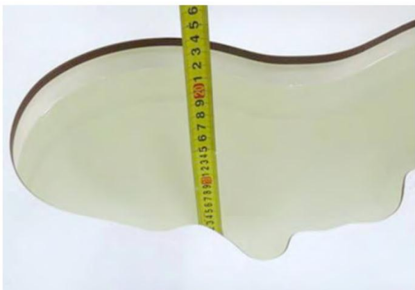
Liquid depth in the head phantom (1750MHz)
