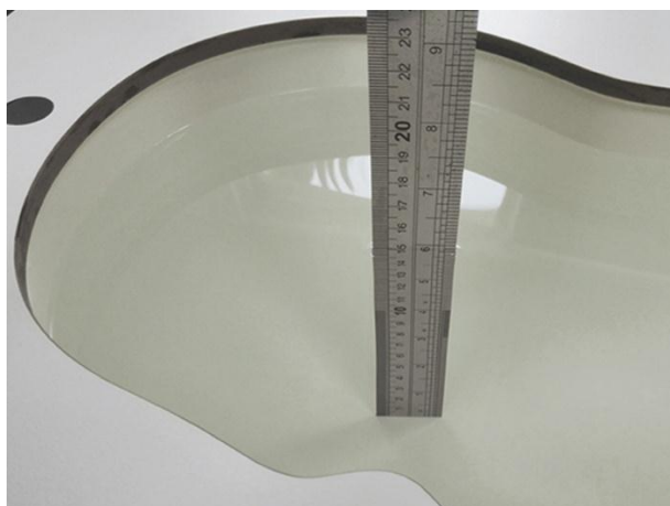
Liquid depth in the head phantom (2450MHz)
