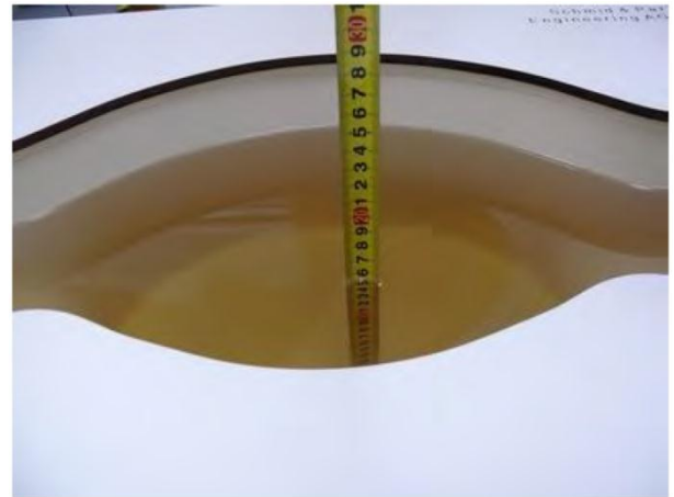
Liquid depth in the body phantom (835MHz)
