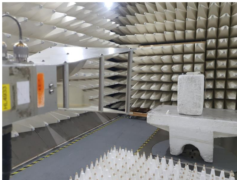
Photograph No.3 Spurious emissions measurement setup in the anechoic chamber in 1 -18 GHz
