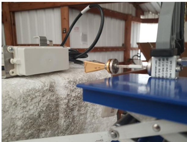
Photograph No.6 Spurious emissions measurement setup at the OATS above 40 GHz, 0.5 m test distance
